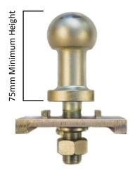
The towball must have a minimum of 75mm in overall height, and have a flat section on the underside of the ball. Towballs that do not meet this criteria will result in the clamp mechanism engaging incorrectly leading to either coupler damage, or an insecure carrier.
